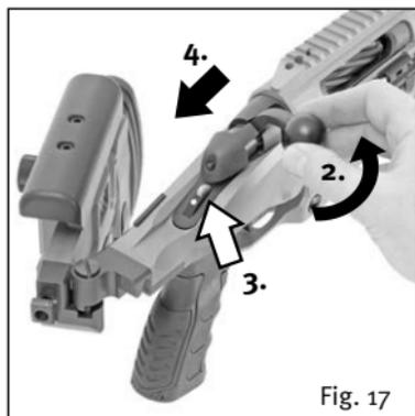
2. Turn the bolt handle  $70^{\circ}$  to the left with your right hand (unlocking).
