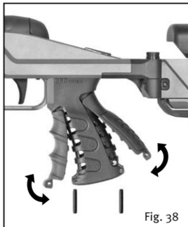
For replacing the frontstrap or backstrap push out the pins with pin punch 3 mm. Swivel out the straps. Assembling in reverse order.
