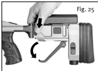
1. Push in push button, clamping lever safety until the clamping lever is released with your right thumb.
