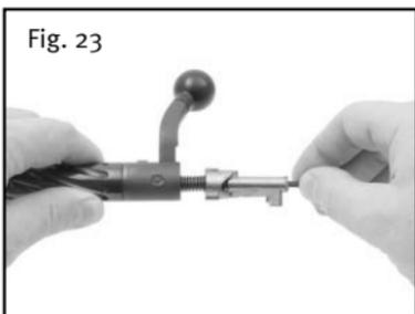
If necessary you can clean and oil all parts of the bolt complete. Any further disassembly should be done only by adequately trained and skilled personnel (gunsmith).
