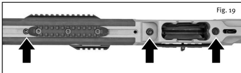
Complete disassembly of the rifle by the user is not required. The three screws at the bottom side of the rifle connect the receiver and the tubular stiffener to the forend of the stock group.
