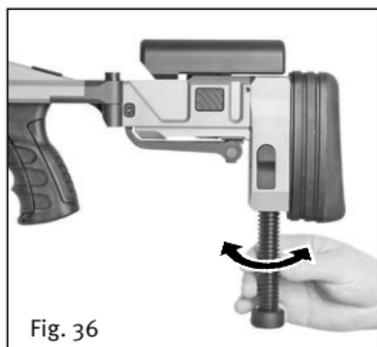
Additional the shaft can be extended up to 30 mm / 1,2" by turning out the spike.
