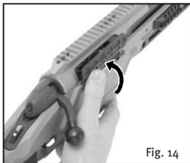
5. Swing dust cover, ejection port upwards with your right thumb until it engages.
