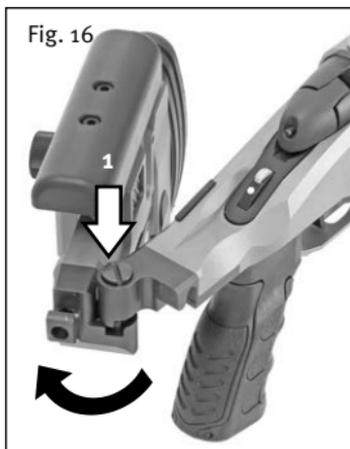
1. Hold the weapon with your left hand and push down the button completely with your right thumb. Swing the stock to the left.
