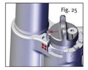
**Position LV:** The Low Velocity (LV) setting is for firing sub-sonic ammunition with a suppressor. DO NOT fire the weapon in this setting with super-sonic ammunition and a suppressor as it may damage the firearm.
