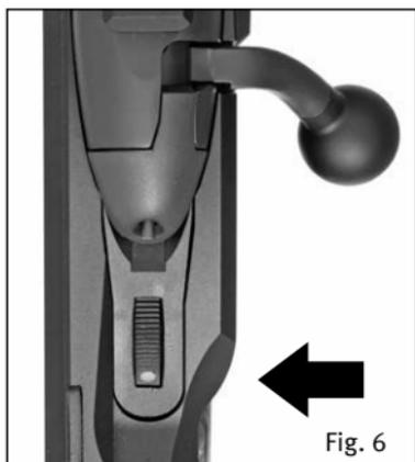
The safety can be operated only when the weapon is cocked or the bolt handle is open! The „2 + 1 positions STEYR ARMS safety“
