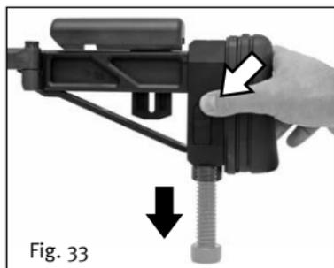
The spike can be adjusted in height to meet the shooter's individual requirements.
