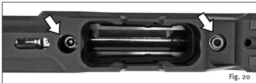
If these screws are loosened, they have to be retightened again with a torque wrench (7 Nm).
