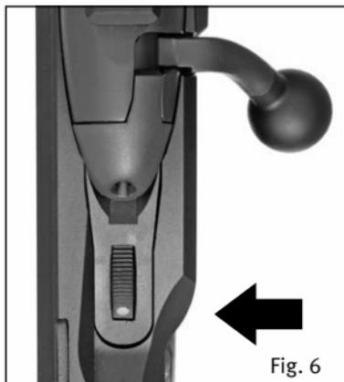
Release safety only shortly before firing the shot. If the weapon has to be reloaded after firing a shot, the bolt handle must be opened.
