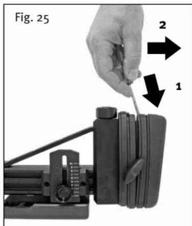
The butt plate can be removed using a screw driver.
